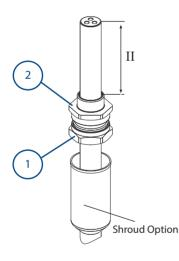
Allow sufficient length of cable, II, to suit equipment. If required, fit shroud.
