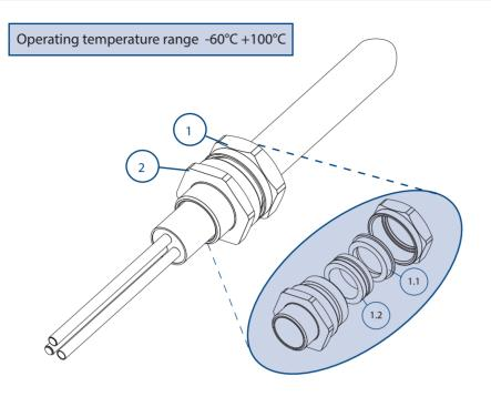
**Certification Details** Gland Type: 121 IP66 Industrial EN 62444 Certificate of Assessment: CML 15CA932-2 1. Backnut 1.1 **Compression Spigot** 1.2 Seal Entry 2.
